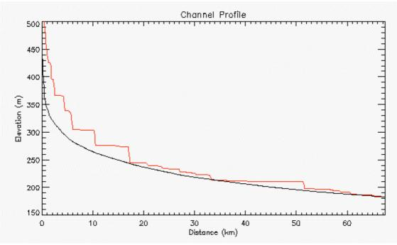
Figure 1. Comparison of main-channel elevation profiles before and after the profile-smoothing operation.
